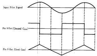
a rectangle wave with a phase of 90° advanced as compared with the input pilot signal will appear as indicated in the right figure b.
