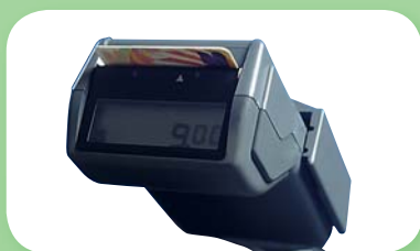
VHB tape was used to bond the IU unit to your car's windscreen.
