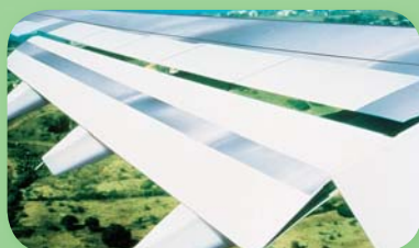
VHB tape holds stainless steel scuff strips to aluminum Airbus A-310 wings strongly.
