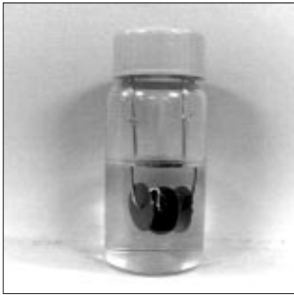
Figure 3 - A glass container with 10ml of artificial sweat solution. Three submerged disks are attached to platinum wire through center holes
